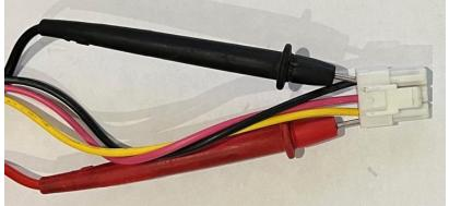
This method ensures a better meter connection to the windings. It also protects the integrity of the plug / socket connections. If testing from the other side of the plug, most likely the meter leads will damage the size of the connectors. An ohm reading across U - V, V-W, and U - W should be between 12 - 14 ohms. If outside of this range, condemn the motor. If an ohm reading difference between any two of the windings is greater than 0.3 ohms, condemn the motor.
