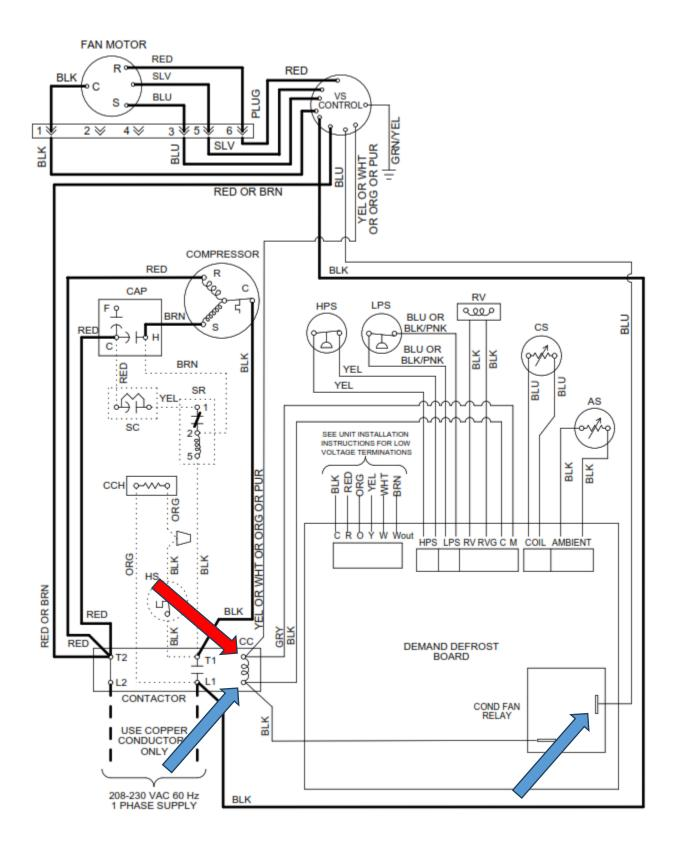
Most premium air conditioning and heat pump models utilize a variable speed outdoor ECM fan motor. The ECM motor controller is provided with a PWM (pulse width modulating) signal in lieu of 24V A/C. The PWM signal can be checked if a digital multimeter capable of reading such signal is available. Check the PWM signal at the locations shown below.
