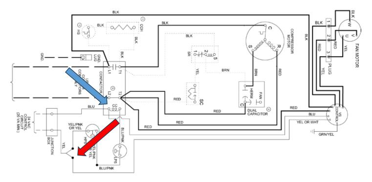
On non-premium heat pump models, the ECM motor controller 24V signal passes through the unit defrost control. The defrost control fan motor relay is normally closed. The fan motor relay only opens during a defrost cycle. When testing, control voltage needs to be tested going into the relay and coming out of the relay.
