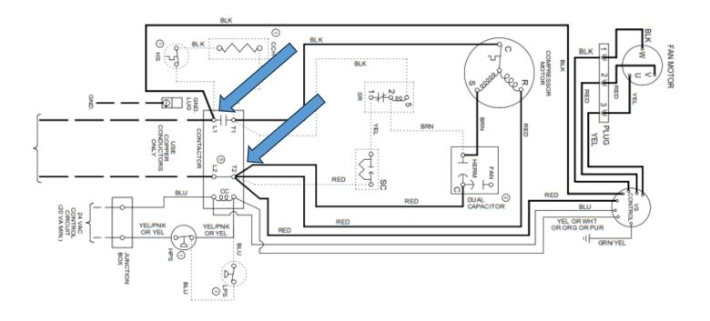
Next test is to check the control signal input to the motor controller. This must be done with an active cooling call. On a non-premium air conditioning unit, the motor controller control voltage input is typically wired in parallel with the outdoor unit compressor contactor low voltage. Test for 24V A/C at the locations shown below.
